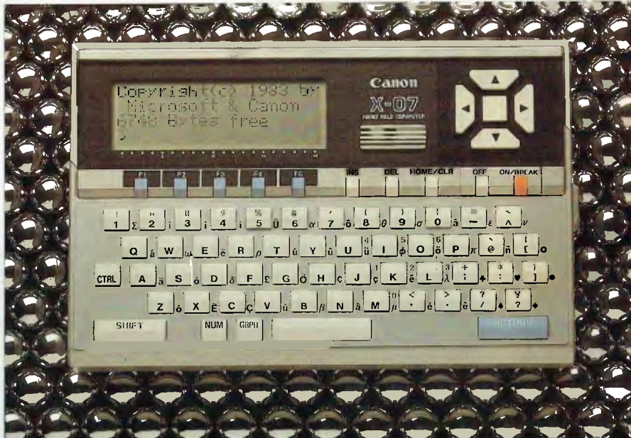
Possibly the smallest micro on the market, the Canon X-07 runs on four AA penlight batteries.
